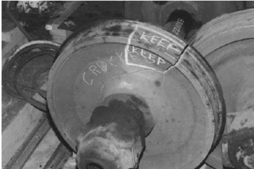
Figure 34 – Cracked or Broken Web
