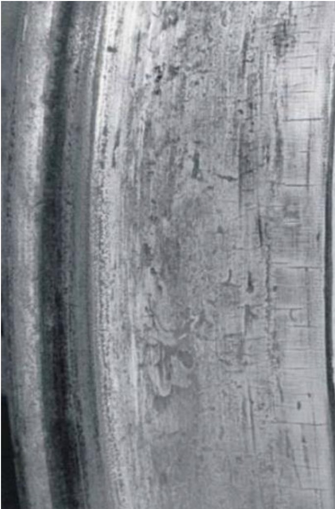
Figure 28 – Class 4 Thermal Crack
