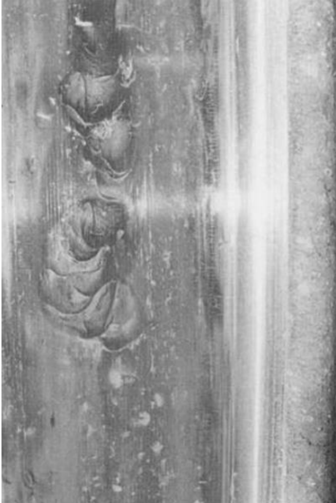
Figure 19 – Class 3 Skidded Wheel – (Multiple Class 2 skids)
