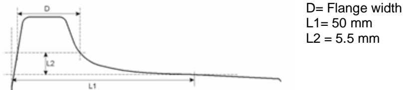
Figure 5: Configuration for flange width measurement
