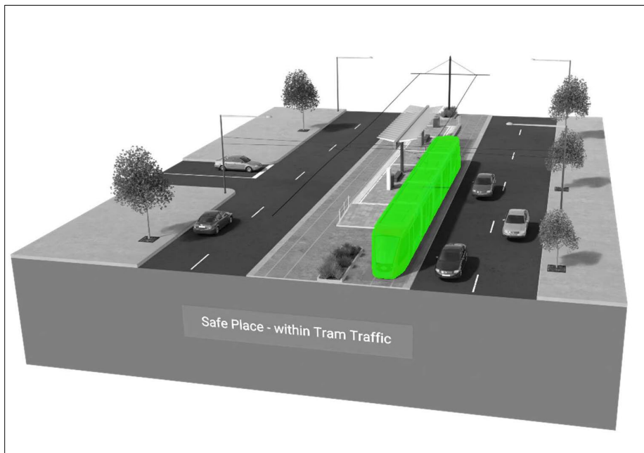
Figure 5: Example of a Safe Place within Tram Traffic
