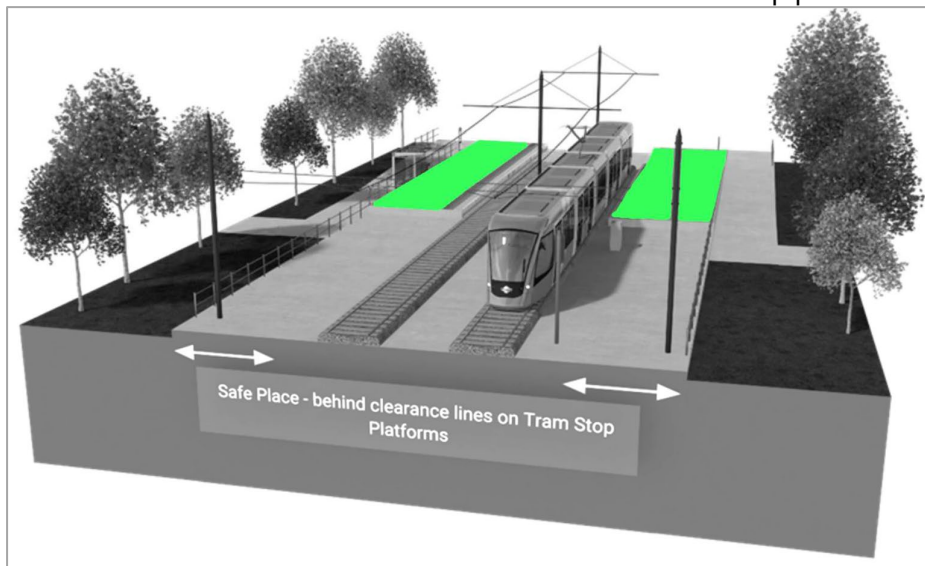
Figure 3: Example of Safe Places on Tram Stop Platforms – Closed Tram Corridor
