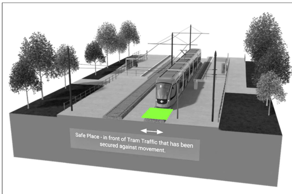
Figure 6: Example of a Safe Place immediately in front of stationary and secured Tram Traffic
